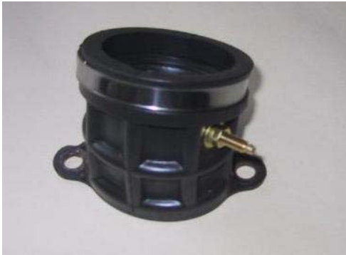
Inlet Manifold with Universal Spigot fitted
