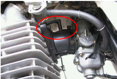
Vacuum connection made in inlet manifold
