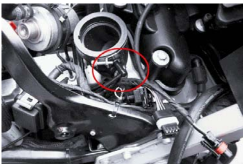
Airbox & throttle body removed, vacuum connection made in inlet manifold
